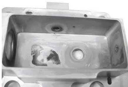
Photo of our Signet 40-3340 Arc Chamber after 844 hours.
