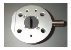
Pictures above is the 30-5395-7 with the replaceable graphite insert. It can be replaced with out removal of the entire assembly.
