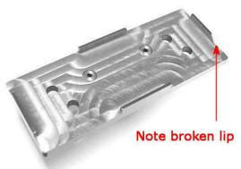
The original OEM design pictured above uses a 3/8" thick tungsten base plate that was extensively machined leaving four fragile lips to locate the side and end plates. These lips are prone to breaking in use and during maintenance and handling.
