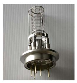
Signet 30-0094R Rebuilt Nude UHV Ion Gauge tube
