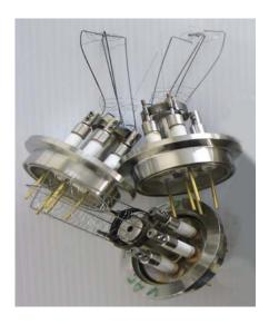
Our rebuild service includes chemical decontamination, all new parts are then attached to the used flange. This process restores a spent gauge to its original functionality which is the same as a brand new gauge.
