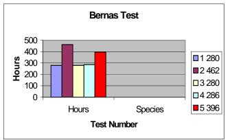
A customer supplied the data above and it is typical of the results obtained in his production operation. This data is for gas only conversion. The Signet Bernas conversion is available in a gas only or gas and vapor inlet configurations. The gas only conversion is Signet Products kit 1088A.
